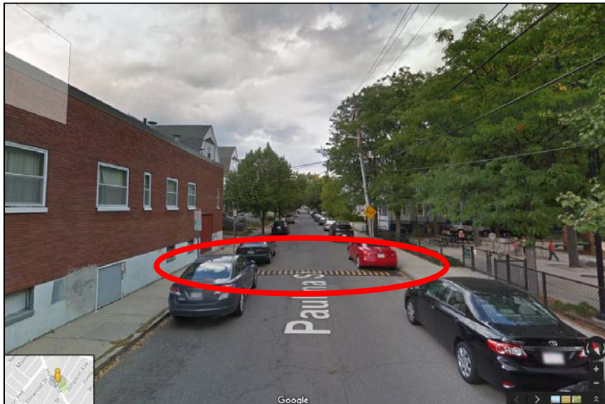
Temporary Speed Hump
